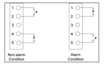
Schematic of contact closures for alarm and non-alarm modes
